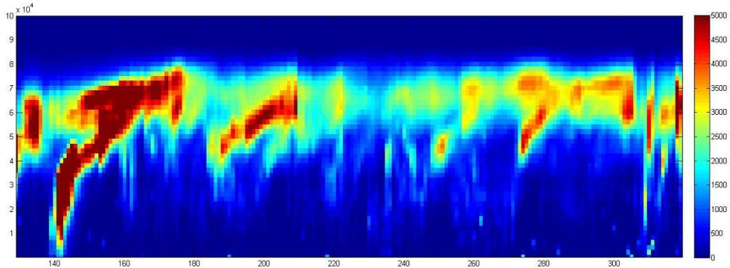
*concentration of particles (color code) as a function of the time for different particle mobility diameter (y-axis) as measured by DPMS*
