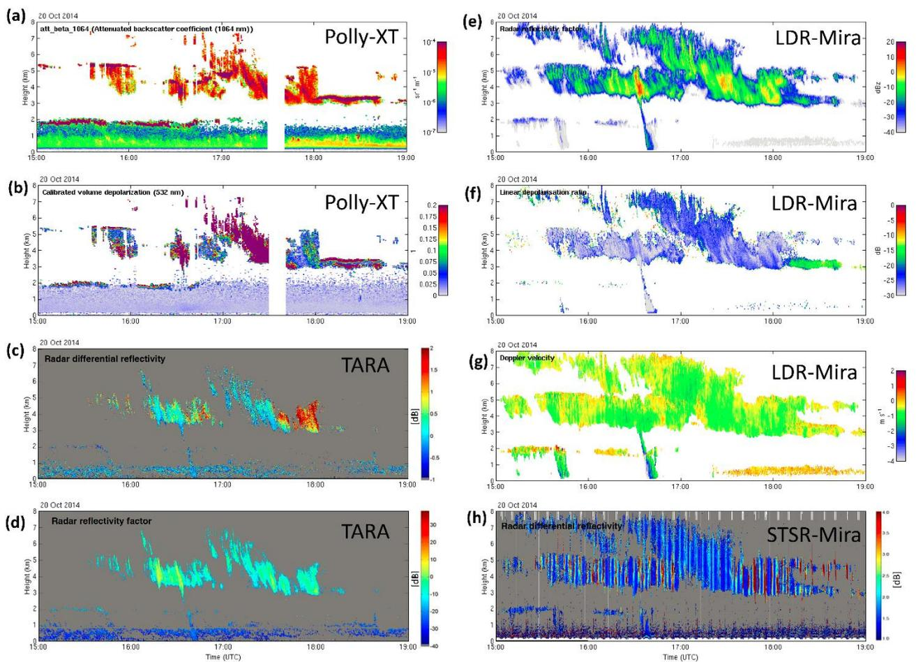
Figure 2 : Combined measurements of a mixed-phase cloud system with the lidar Polly-XT (a,b), 3-GHz radar Tara (c,d), LDR-mode cloud radar Mira (e-g), and STSR-mode cloud radar Mira (h) on 20 October 2014 from 1500 to 1900 UTC.
